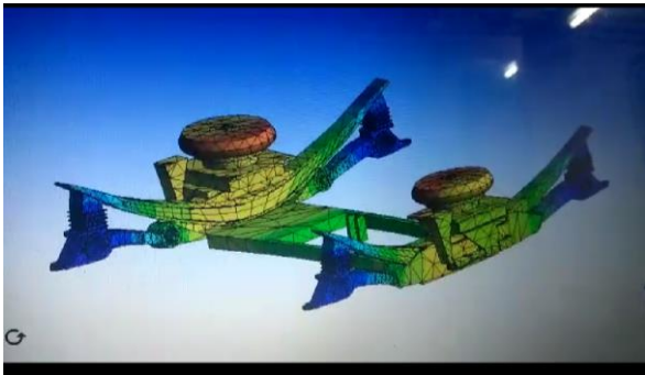
Figure 5: Equivalent Stress in EMU BOGIE
